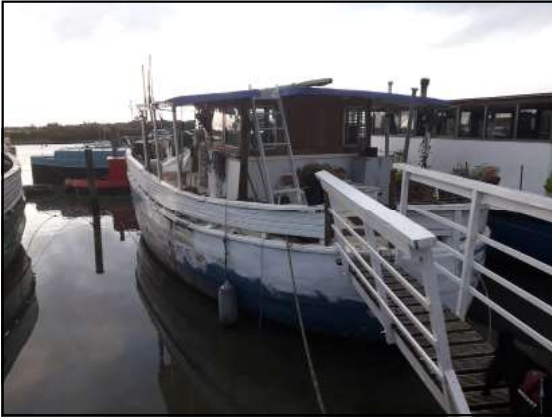
Monbretia is an MFV (motor fishing vessel) built in 1942. Grant is engaged in a long-running project to replace her larch planking.
